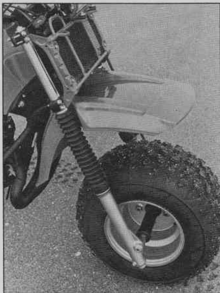
Ten-inch wheels are a radical departure from the norm. Stiff sidewalls on tires make for precise steering.
