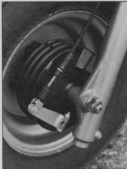
Front drum brake is not as good as Honda's disc but still manages to stop the KXT.
