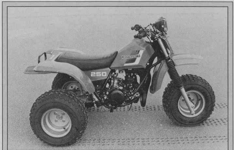
Single-strt Uni-Trak is a dead ringer for the motorcycle version. Rebound damping is adjustable.
