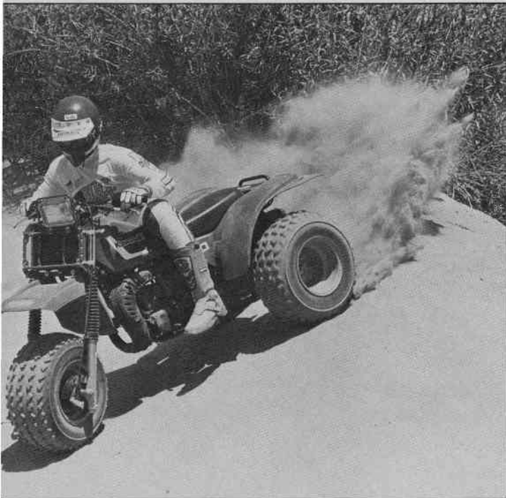
The KXT is a very stable slider, due mostly to the firm-walled low-profile tires and 10-inch wheels.
