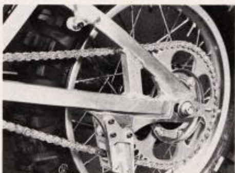
A dished rear sprocket ring prevents a derailed chain from becoming lodged between the sprocket and the swing arm.
