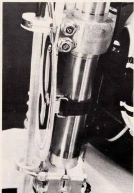
Knurled sections on the tubes give the aluminum triple clamps an improved grip.
