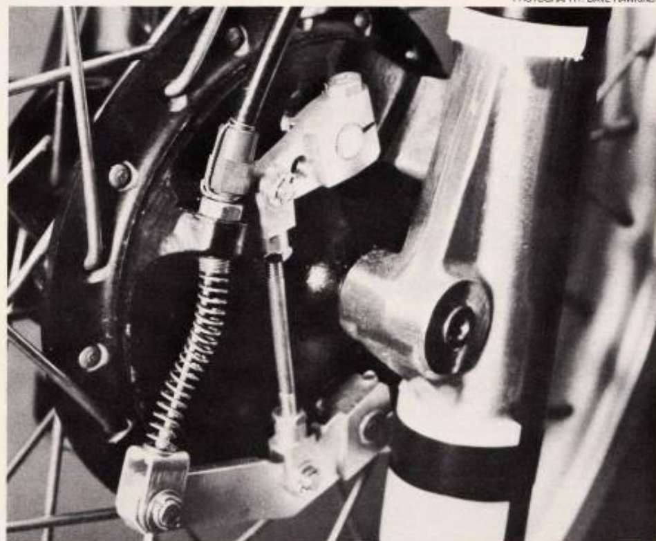
The diminutive conical front brake belies its stopping strength. Instead of the traditional leading/trailing configuration, powerful double leading shoes are used.
