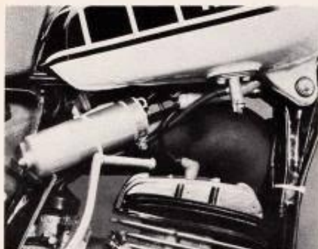
Yamaha's works head closely resembles the 125 Honda's quasi-radial head.
