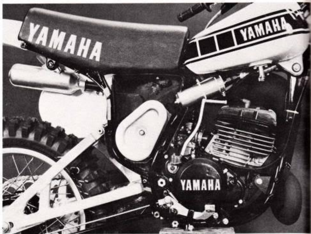
At 202.5 lbs. the works bike is almost 30 pounds lighter than the stock YZ-F. Heavy rims and steel shift lever and screws could be replaced to further lighten the bike.
