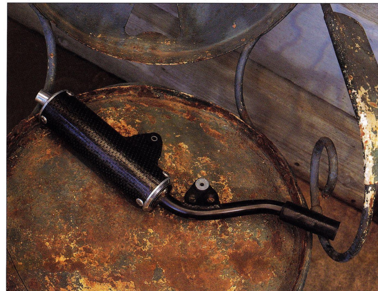
The factory 80's carbon-fiber silencer was built by Go Kart specialist Randy Blevins of Riverside, California. It's a carbon-fiber extrusion with aluminum end caps wrapped around a standard KX80 silencer core.
