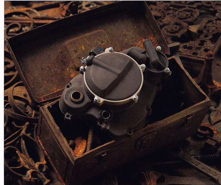
The factory bike's immaculate quick-change clutch cover was fabricated from a stock component by legendary minicycle builder Dave Miller. A pair of machined-aluminum mounting rings seal with an internal O-ring. The finished components are anodized for a works look.
